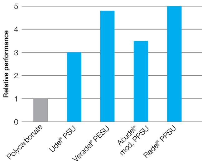
Figure 4 shows a comparison of the hydrolytic stability of these resins with polycarbonate and PSU. The hydrolytic stability of Udel® PSU is excellent and surpassed only by Radel® PPSU and Acudel® mod. PPSU.
