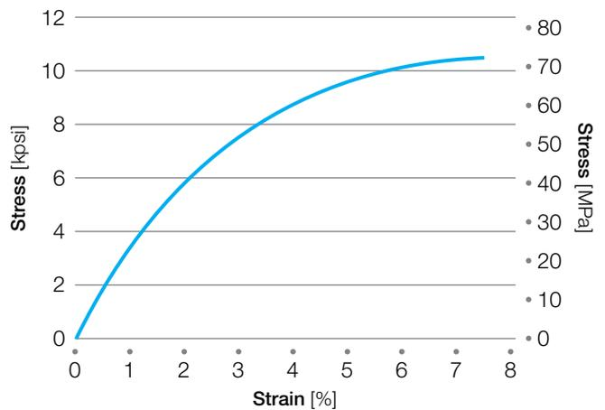
**Figure 11:** Acudel® 22000 stress-strain curve to yield
