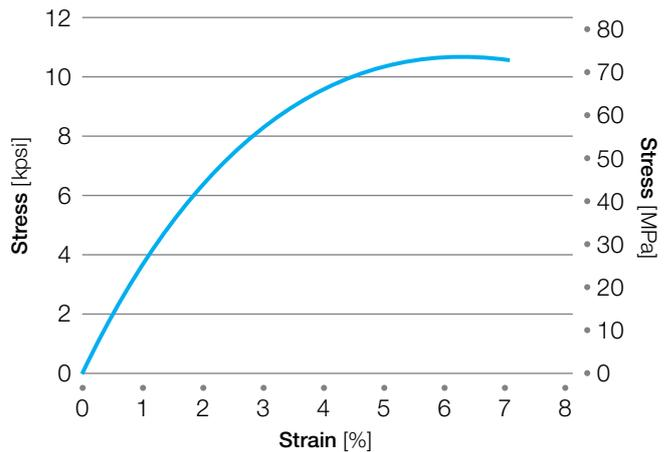
**Figure 12:** Veradel® AG-320 stress-strain curve to break
