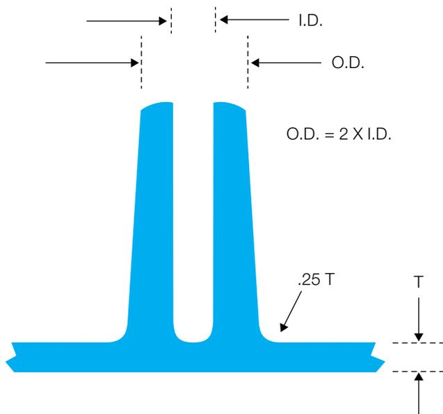
Additional forces imposed on a boss may be transmitted down the boss and into the nominal wall. For this reason, a minimum radius of 25% of the wall thickness is required at the base of the boss to provide strength and reduce stress concentration. A boss can be further strengthened by using gusset-plate supports around the boss, or attaching it to a nearby wall with a properly designed rib. Heavy sections should be avoided to prevent the occurrence of sink marks on the surface of the part.
