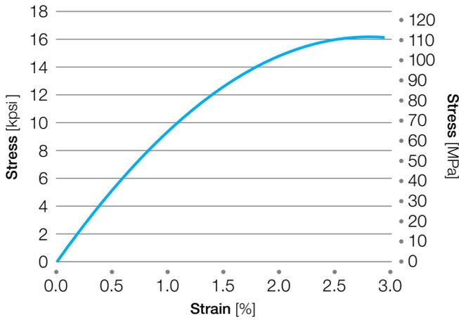
**Figure 13:** Veradel® AG-330 stress-strain curve to break
