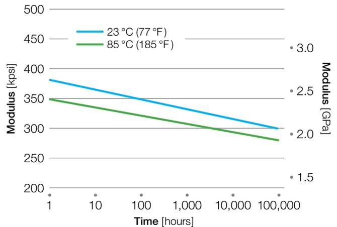
The creep modulus data for Radel® PPSU are shown in Figure 28. Radel® PPSU resin has surprisingly good creep resistance, especially at elevated temperature.
