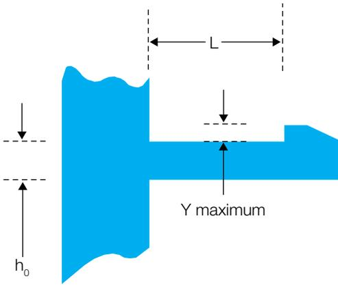
**Figure 73:** Snap-fit design using tapered beam
