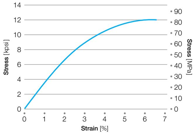
**Figure 10:** Radel® R-5000 stress-strain curve to yield
