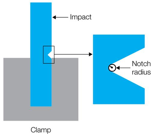
As shown in Figure 23, Radel® PPSU exhibits exceptional impact resistance by the notched Izod method. While Udel® PSU and Veradel® PESU are generally considered to have good impact resistance, the impact resistance of Radel® PPSU is an order of magnitude higher.
