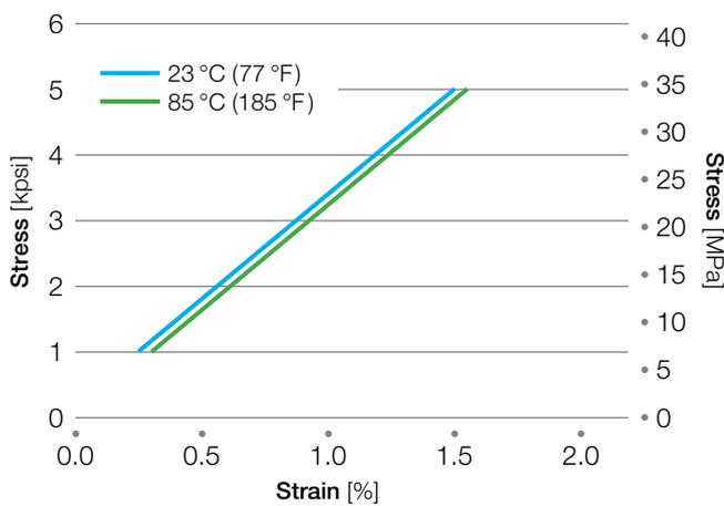
**Figure 30:** Isochronous stress-strain curve Radel® R-5000 at 100 hours
