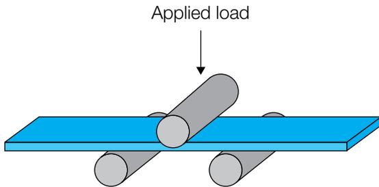
Flexural testing provides information about a material's behavior in bending. In this test, the bar is simultaneously subjected to tension and compression.
