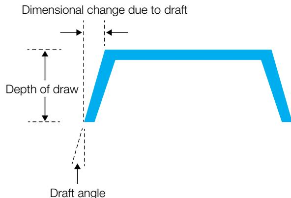
Adequate draft angle should be provided to allow easy part removal from the mold. Generally, the designer should allow a draft angle of 1° to 2° per side for both inside and outside walls for sulfone resins. In some special cases, smaller draft angles have been used with draw polish on the mold surface.
