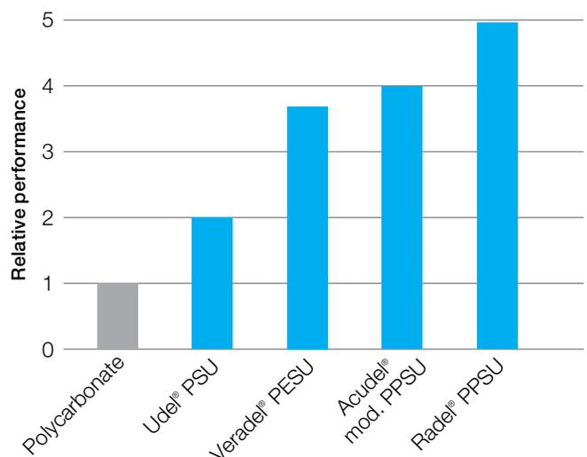
A key property in many applications is impact resistance, which is a difficult property to quantify. Some tests measure notch sensitivity and others measure resistance to high-speed penetration. Figure 6 shows an estimate of the practical impact resistance of Radel® PPSU resin which includes drop impact ratings as well as tensile impact results. The Figure shows that these resins are tough, ductile materials and they all have excellent practical impact resistance.
