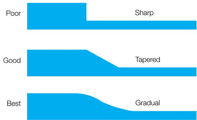
Also, from a structural standpoint, a sharp transition will result in a stress concentration, which may adversely affect part performance under loading or impact.
