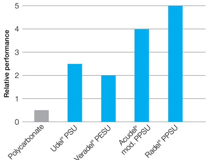
The relative performance of the Radel® PPSU and Veradel® PESU resins when exposed to organic solvents is shown in Figure 5. The graph shows that Radel® PPSU has by far the greatest resistance to attack and/or stress cracking from organic solvents. Veradel® PESU, Acudel® mod. PPSU, and Udel® PSU are clearly better than polycarbonate.
