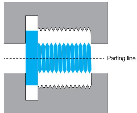
Besides female threads, inserts can be threaded male styles, locating pins and bushings. The recommendations on installation procedures and boss dimensions can be provided by the insert supplier and resin manufacturer.
