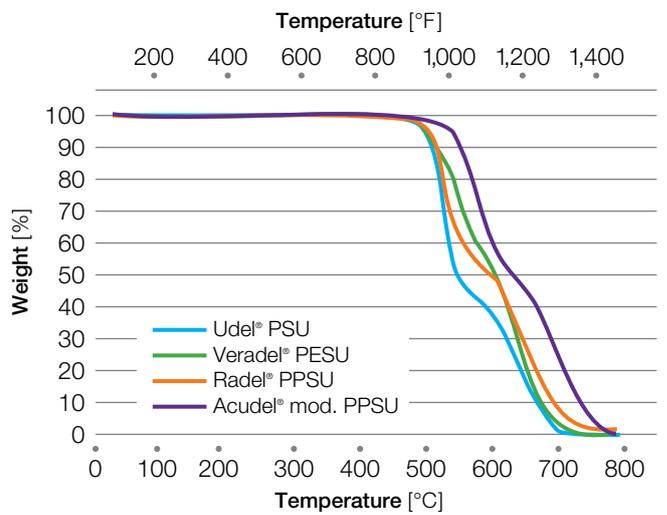
Table 21 gives the temperature at which the listed weight losses were recorded. These data clearly show that Radel® PPSU has the best thermal stability of the resins tested.
