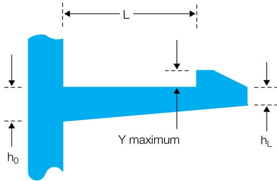
**Figure 74:** Proportionality constant (K) for tapered beam
