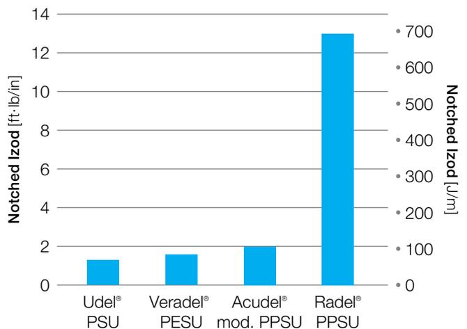
Failure of a material under impact conditions requires that a crack form, then propagate through the specimen. In the notched Izod test, the notch acts like a crack and the test is primarily measuring crack propagation resistance. When the test is run without a notch, a crack must first be formed, then propagate. Sulfone polymers are extremely resistant to crack formation, as evidenced by the fact that none of the neat resins break in the un-notched test.
