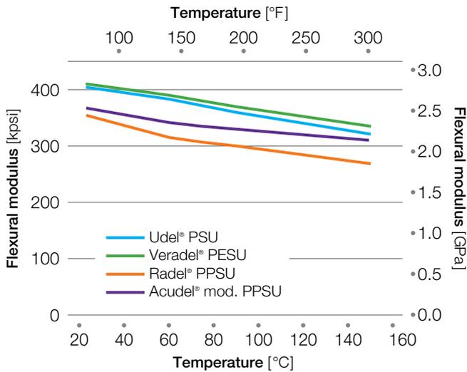
Of the three sulfone polymers, Veradel® PESU has the highest initial modulus and also the highest modulus at elevated temperature.
