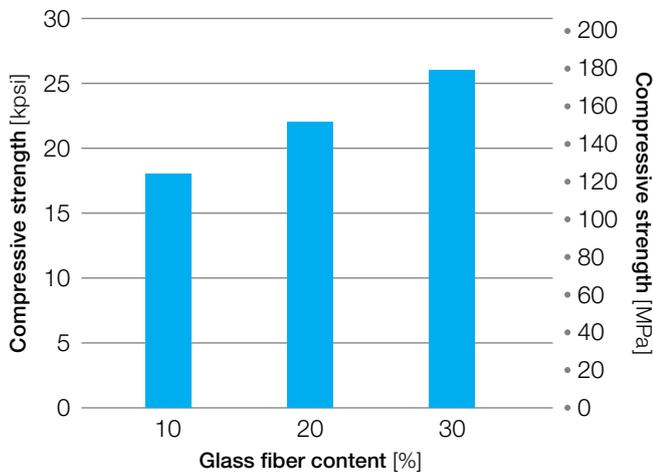
**Figure 20:** Compressive modulus of glass-filled Veradel® PESU
